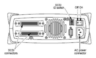
**Figure 1-5** External tape drive: back-panel components
